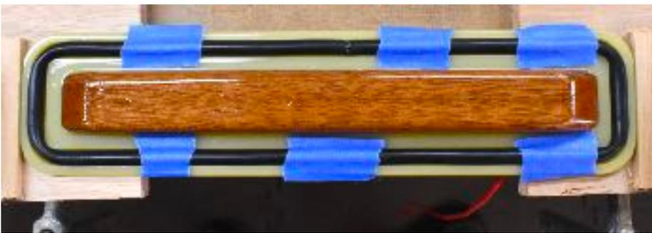
Practice putting the cap in place & dogging it down before lifting one end of the gasket, applying glue, getting the gasket back in place and quickly placing the cap and dogging it down.
