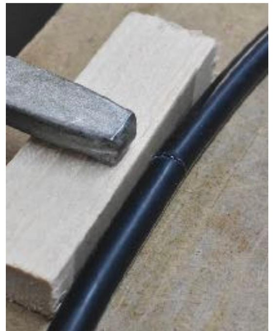
Now is when the fun begins. Re-install gasket and tape down as shown. **The lid will be used for pressure as the glue dries**, so try installing it and dogging it down. Add more tape if necessary to keep the gasket in the notch.
