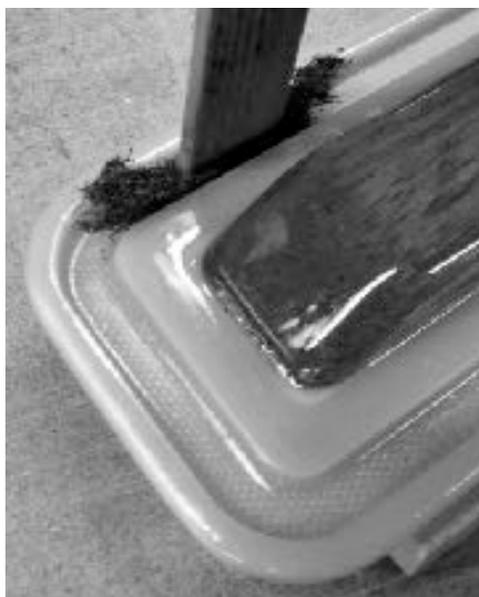
**All 3 gasket notches should be prepped for gluing with multiple narrow strips of scrubbie.**
