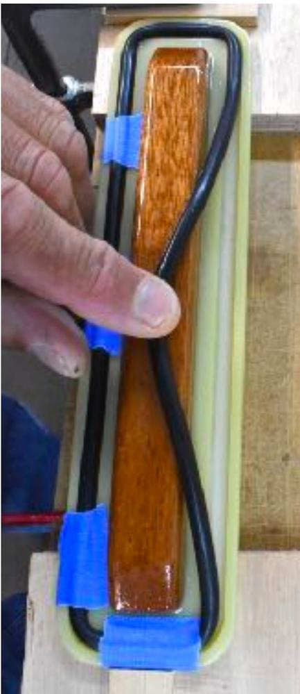
**Firmly tape the far end & pull up & glue one edge at a time, dogging the cap down each time.** (photo on left).
