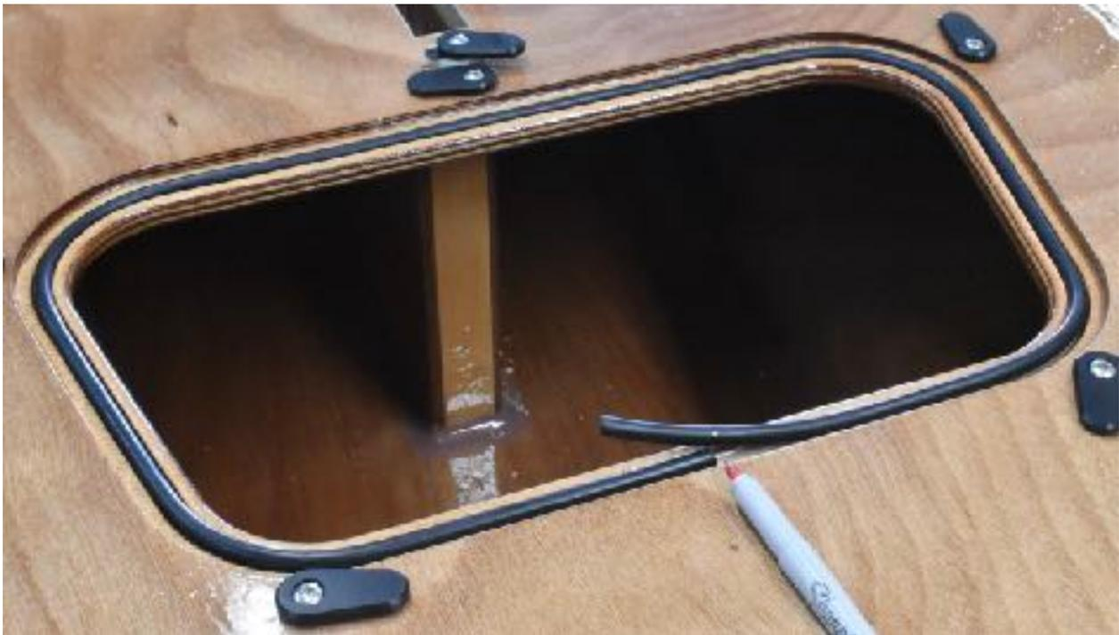
Both the foredeck and trunk cap gaskets need to be butt-glued to make a loop before installing. This should be done by **applying a thin film of cyanoacrylate to one end** and pushing the ends together in an inside corner as shown.
