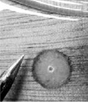
Drill the holes for the screws as square as possible to the surface of the foredeck and use a countersink to lightly bevel the edges of the holes.
