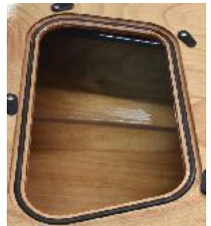
The trunk cap gasket is easier, but should still be glued in small steps.
