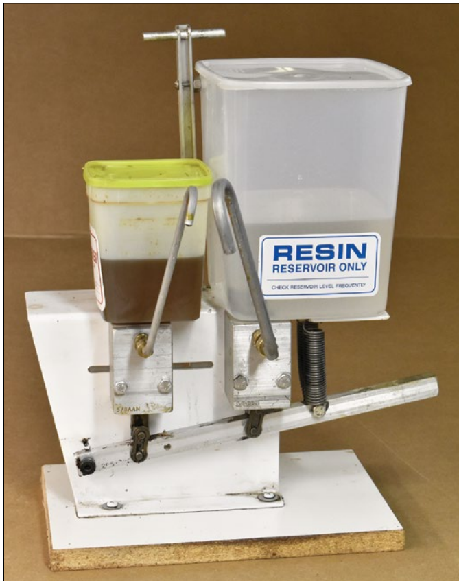
A positive-displacement pump draws from separate reservoirs of resin and hardener with the stroke of a single lever.
