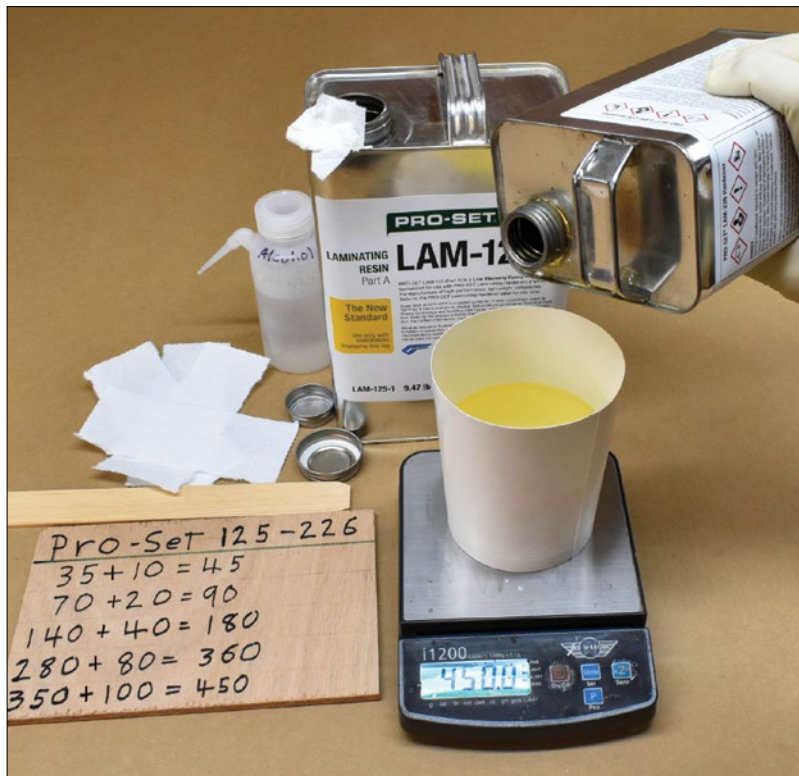
Metering with a digital scale can be faster by referring to a list of batch sizes for each epoxy and mixing ratio the shop uses.
