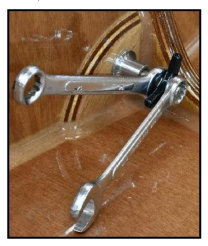
Put two nuts together on either end of the pin and tighten them together very tightly with the wrenches. (photos below)
